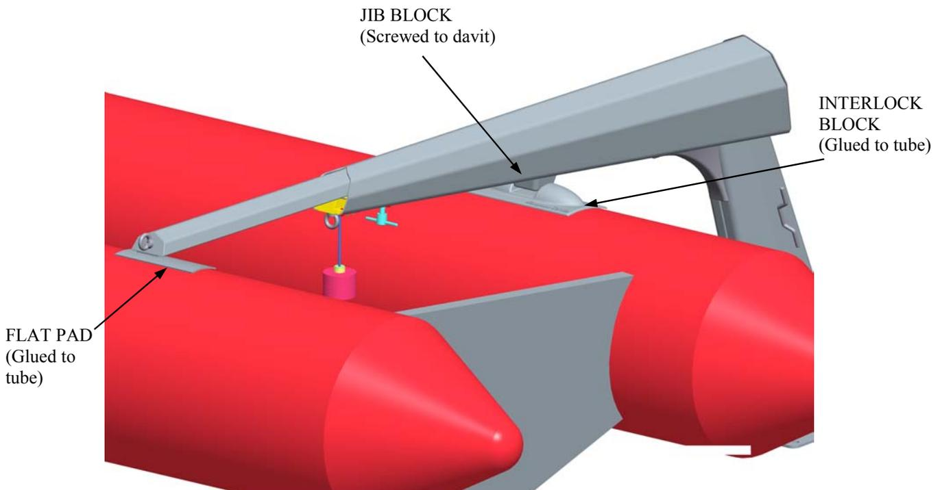
The interlock blocks and flat pads are fixed to the tube by adhesive. The fitting position can be easily marked on the dinghy when it is raised in the davits. The interlock block and pad profiles can then be traced with a pencil on to the dinghy tube.
